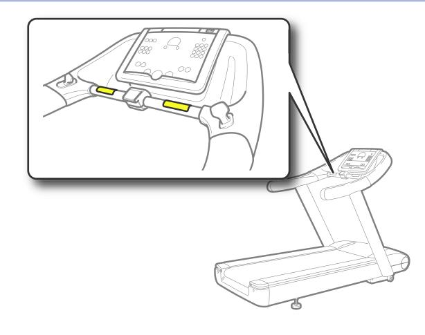
**Central handgrip**: can be held when walking with small strides. It has **sensors** for monitoring the heart rate (hand sensor).
